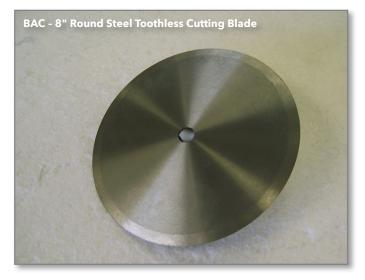
Echo Eliminator panels are made from BAC, bonded acoustical cotton, and do not cut easily with standard tools. Acoustical Surfaces offers this specialized blade that fits a standard table saw that allows on-site alterations to the materials. This ensures the material can be easily manipulated to fit a project, with minimal damage to the product itself. If you are thinking of utilizing Echo Eliminator, don't work without the BAC cutting blade.
